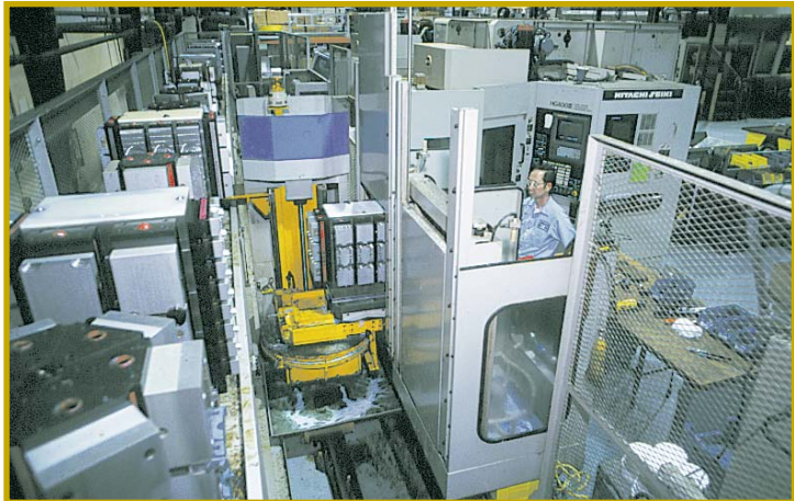
Two-spindle horizontal machining cell, with RGV and 32 pallet stoker system, optimizes spindle time.
